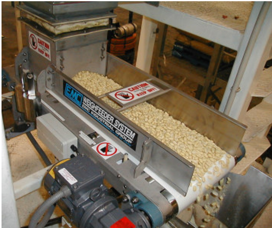
EMC Weigh Feeder controlling the flowrate of nuts into the oven
