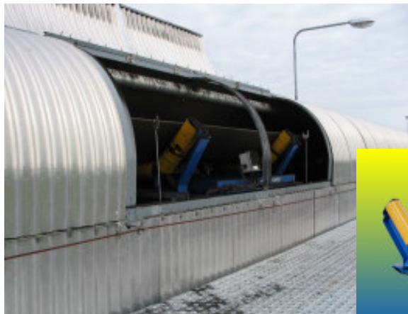
W&M approved EMC B152 Dual Idler Belt Weigher installed on the enclosed load-out conveyor. Inset shows the B152 model.
