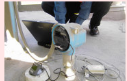
Commissioning the Micropilot M FMR250 with the ToF Tool software package
