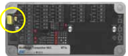
MT4 Transmitter: 4 loadcell terminals, 1 digital input, 2 digital outputs and one 4-20mA output
