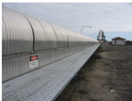
Enclosed coal load-out conveyor system. Picture below shows a train being loaded from the storage hoppers.
