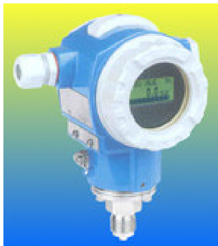
PMC 71 with Ceraphire® ceramic sensor -40 °C to 150 °C, 100 mbar to 40 bar
